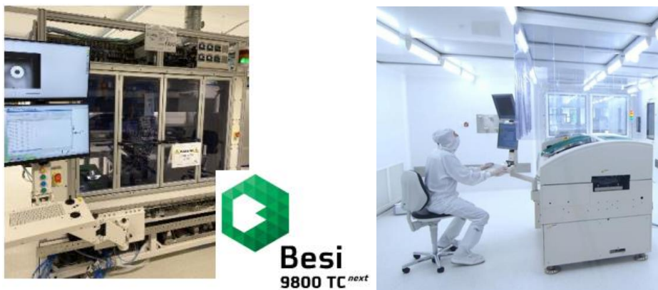
Bron: Besi presentatie CMD 2022, links de thermo compression bonding machine en rechts de hybrid bonding machine
